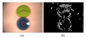
Figure 6: (a) An image of textureless/transparent/reflective objects. (b) Depths estimated by our stereo system. The grayscale value indicates the depth (darker being closer to the camera). Black represents areas where stereo vision failed to return a depth estimate.
