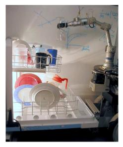
Figure 1: Our robot unloading items from a dishwasher.
