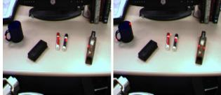
Figure 16: Grasping point classification in kitchen and office scenarios: (Left Column) Top five grasps predicted by the grasp classifier alone. (Right Column) Top two grasps for three different object-types, predicted by the grasp classifier when given the object types and locations. The red points in each image are the predicted grasp locations. (Best viewed in color.)
