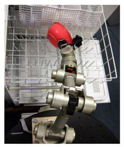
Figure 15: Dishwasher experiments: Failure case. For some configurations of certain objects, it is impossible for our 5-dof robotic arm to grasp it (even if a human were controlling the arm).
